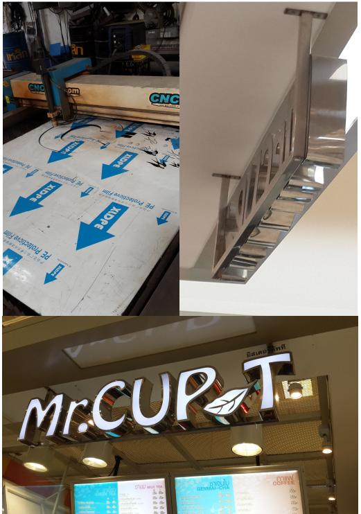
Code: 2014052401-X Process: CNC Plasma / Laser / LED Lead time: 3-4 Days / Size: 0.6 x 2M (Thk: 300mm) Total Cost: 25,000 Bahts (Cutting / Welding / Material / Assembly / Engineering Design) Original Design by Customer Al Files
